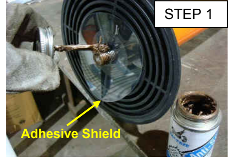
STEP 1 Place the adhesive shield then coat threads with anti-seize compound.
